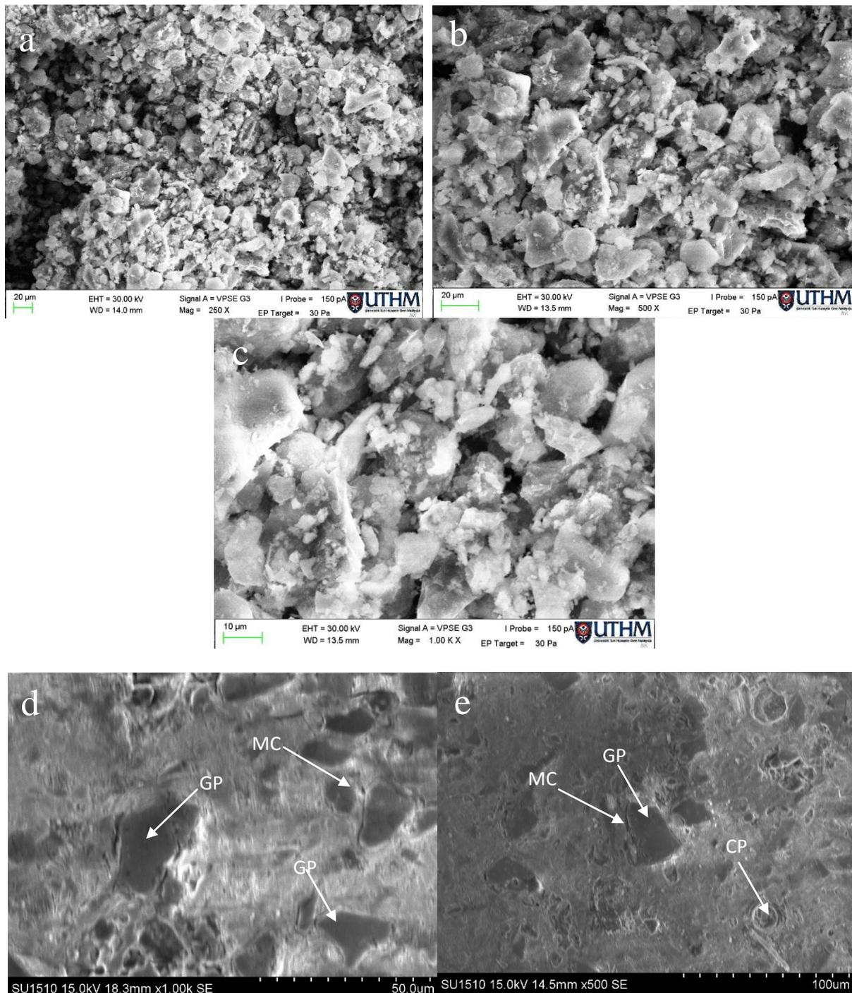
**Figure 1.** SEM of POFA powder (a,b and c) and porcelain without addition of ferum  $\text{Fe}_2\text{O}_3$  (d) and after addition (e). [MC = micro crack, CP = closed porosity, GP = Glassy phase] (d) and after addition (e). [MC = micro crack, CP = closed porosity, GP = Glassy phase].
