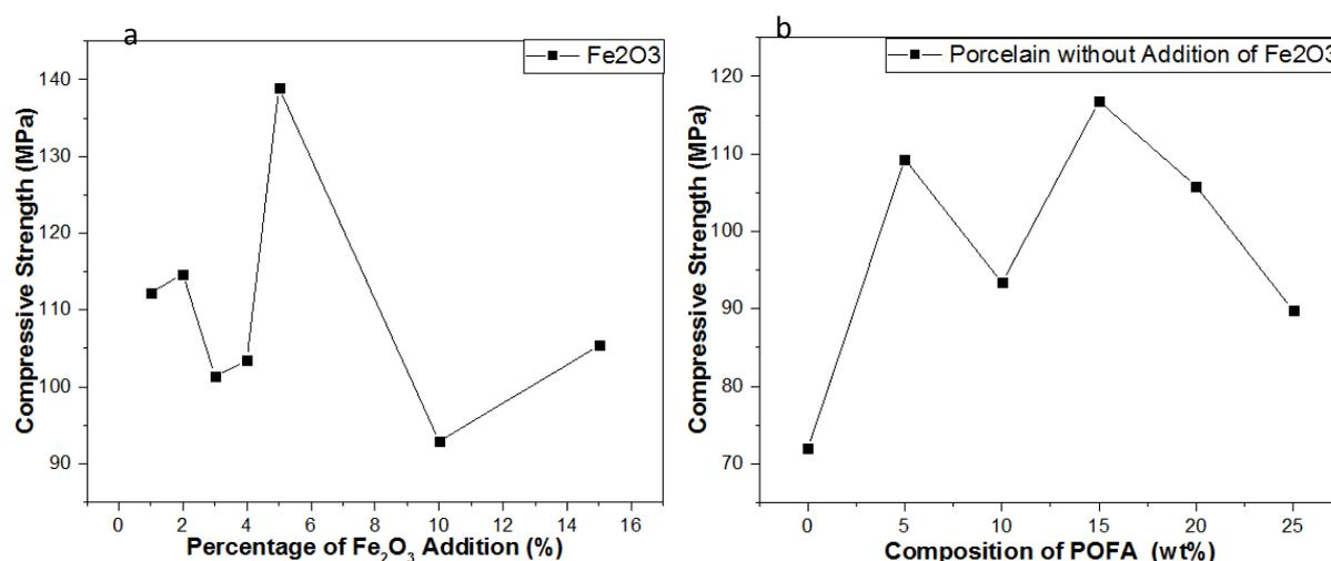
**Figure 3.** The compressive strength of porcelain with and without the addition of  $\text{Fe}_2\text{O}_3$ .
